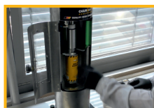
After filling open the door and extract can.
