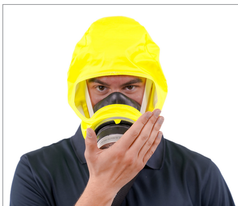
Check the fit of the half mask by closing the front filter opening with the palm of your hand. Breathe in.
