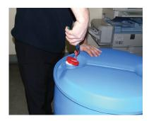
Before starting, visually examine the drum – are the sides 'ballooned' out or 'pinched in' (this effect is known as 'panelling'). Any of these symptoms suggests that there is a slight positive or negative pressure in the container, Using pliers or some other suitable tool, remove the tamper-evident seal.
