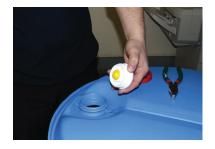
The shroud has a perforation approximately 1 millimetre in diameter – this can get blocked with dried liquid
