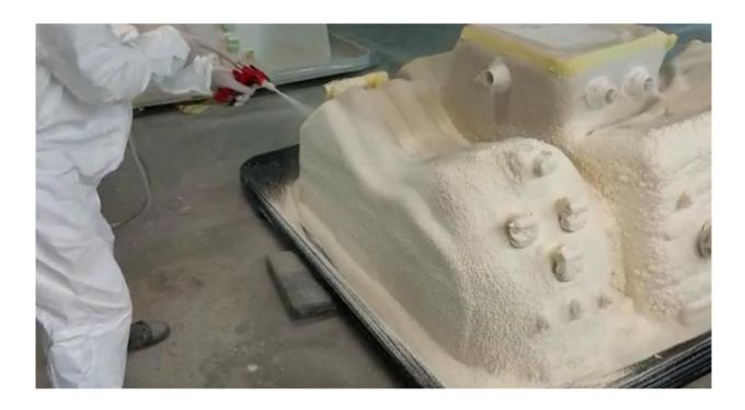
MAXTWO closed cell foam is used as insulation material for hot tubs.
