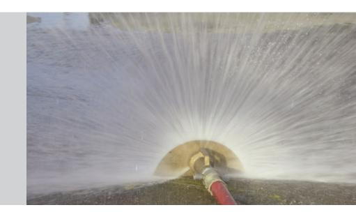
The Angus Fire HYDROshield directs the flow of water into a flat fan shape. The fan, or water curtain, is used to protect fire fighters from smoke, flame, radiant heat and to stop the flow of gases at ground level.
