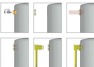
**Warning:** Before any cutting work is done to the tank shell, which could cause sparks and hot spots, it must be ensured that the tank is empty and purged of any flammable vapours.
