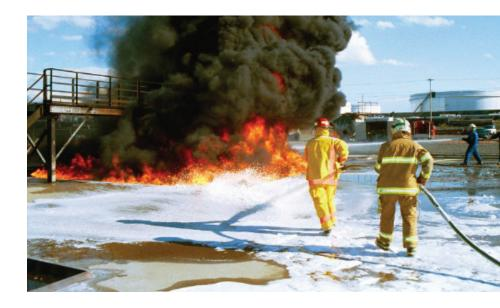
Tridol<sup>c6</sup> ATF C 3-6 is a competitive Alcohol Resistant Aqueous Film-Forming Foam (AR-AFFF) concentrate for extinguishing and securing flammable hydrocarbon and polar solvent liquid fires.
