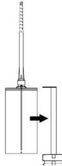
**Note:** The SAF-Q2 nozzle is in two sections. One section contains the mixing elements and the other section is an extension piece. Connect the extension piece to the mixing section by pushing the two sections firmly together until a positive engagement is felt.
