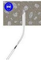
10. Insert the mixing nozzle to the bottom of the hole. Extrude the resin and slowly withdraw the nozzle from the hole. **Ensure no air voids are created** as the nozzle is withdrawn. Inject resin until the hole is approximately ¾ full and remove the nozzle from the hole.
