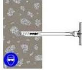
11. Select the steel anchor element ensuring it is free from oil or other contaminants, and mark with the required embedment depth. Insert the steel element into the hole using a back and forth twisting motion to ensure complete cover, until it reaches the bottom of the hole. Excess resin will be expelled from the hole evenly around the steel element and there shall be no gaps between the anchor element and the wall of the drilled hole.
