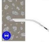
10. Insert the mixing nozzle to the bottom of the hole. Extrude the resin and slowly withdraw the nozzle from the hole. **Ensure no air voids are created** as the nozzle is withdrawn. Inject resin until the hole is approximately  $\frac{3}{4}$  full and remove the nozzle from the hole.
