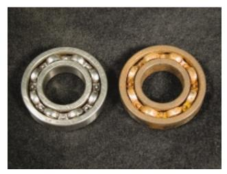
The bearing on the left was treated with CorrosionX; the one on the right was left untreated and both were sprayed with seawater every day for two weeks. Note the remarkable difference.
