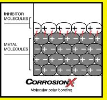
creep through microscopic voids and over surface irregularities to penetrate between seized surfaces where it softens rust and corrosion deposits to free up frozen parts.
