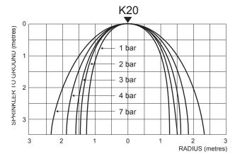
Typical print diameter = 3.9 metres at 4 bar.g. when mounted 2.5 metres above ground
